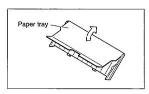
Insert the two fins on the paper tray into the slots on the back of the unit.
