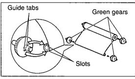
Insert the film into the cartridge so that the blue gear matches the blue label on the cartridge.
